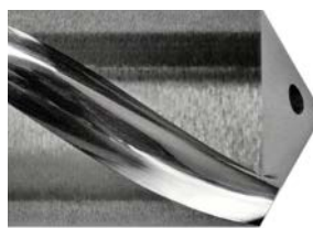
Drill flute polished using STARTEC XP-F Rz = 0.20 µm
